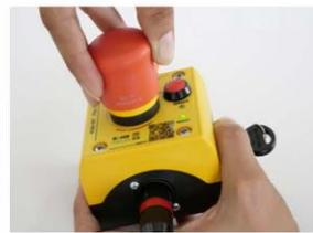
**A:** Release the E-STOP button by pulling it upwards.
