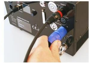
**D:** Use supplied Neutrik powerCON power cable to connect the laser system to a main power supply using the input connector.
