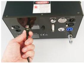
**A:** To control the system with an external signal such as Ethernet or ILDA, plug the corresponding cable into its designated connector at the back of the unit.
