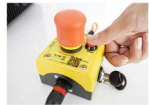
**B:** Press the START button on the E-STOP Remote.
